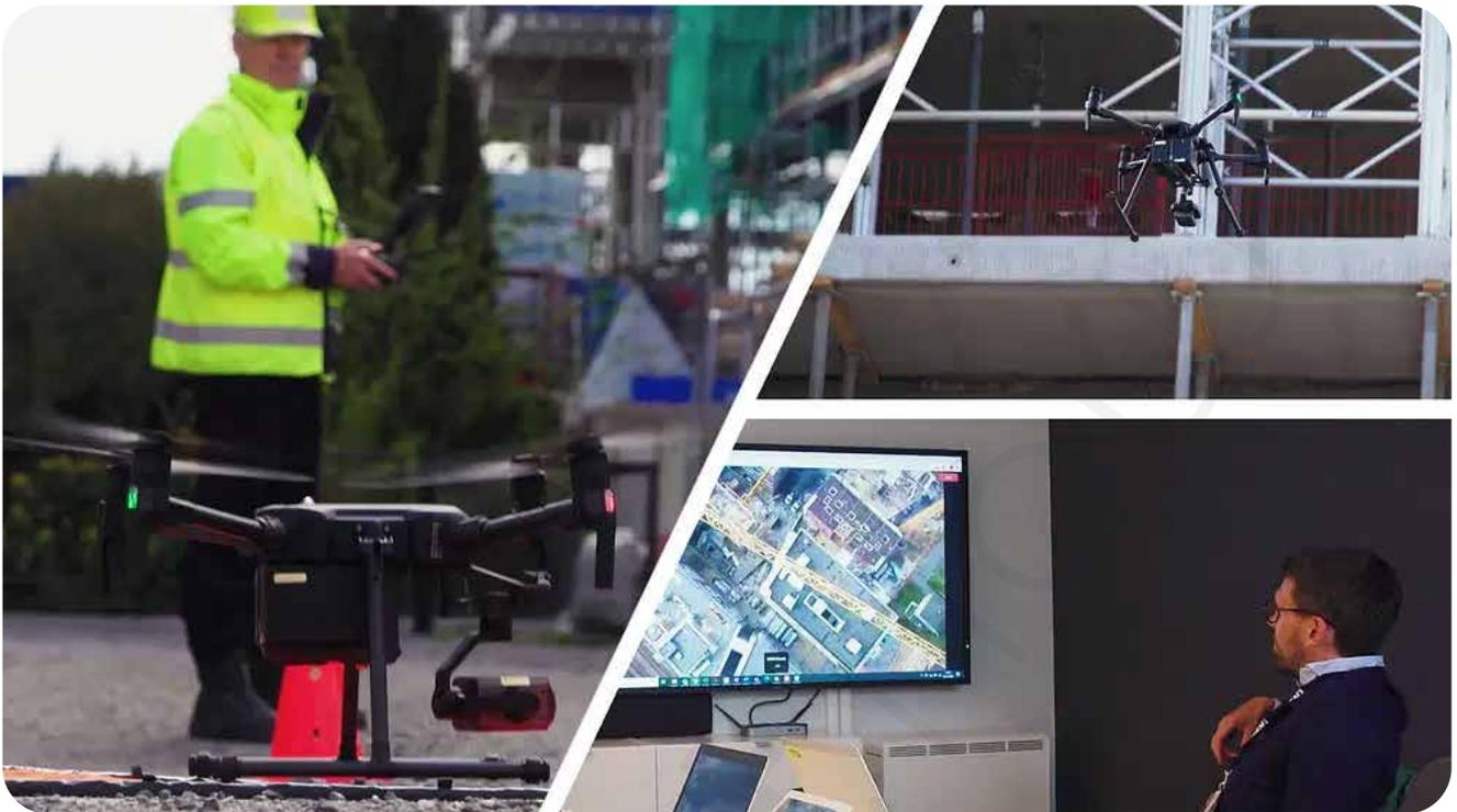
HENT employed the services of one of FlytBase's partners, Droneverkstedet, to inspect the outer facades of one of their residential projects using drones. Jørn W. Howlid, an experienced and certified drone pilot conducted the operation successfully and live-streamed the video using the FlytNow platform over Telia's high-speed 5G network.
